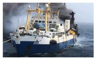
The engine room presents considerable risk, because you here will find pressurized fuels being pumped to engines and hereby meeting hot surfaces, although unintentionally, which may result in the ignition of leaking gasses or oil mist vapours.
